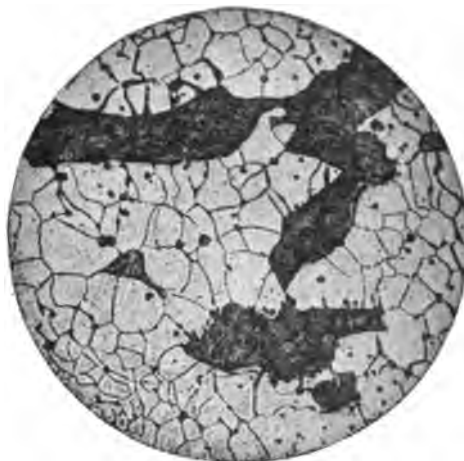
FIG. 14. — Wrought Iron. Transverse Section. Magnification not Stated. (Guillet.)
